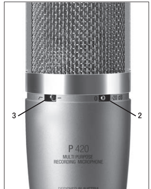
Fig. 2: Preattenuation (2) and bass cut (3) switches on PERCEPTION 420 rear.
